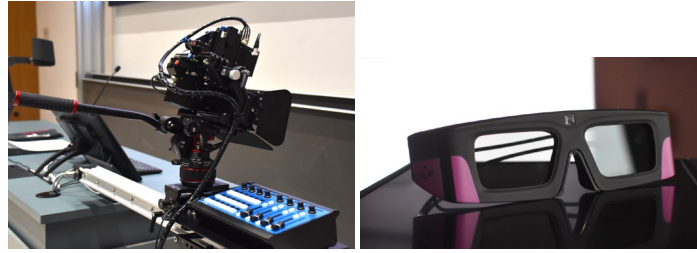
Fig. 2. Left the 3D mirror rig camera – Right active shutter glasses for stereoscopic view
