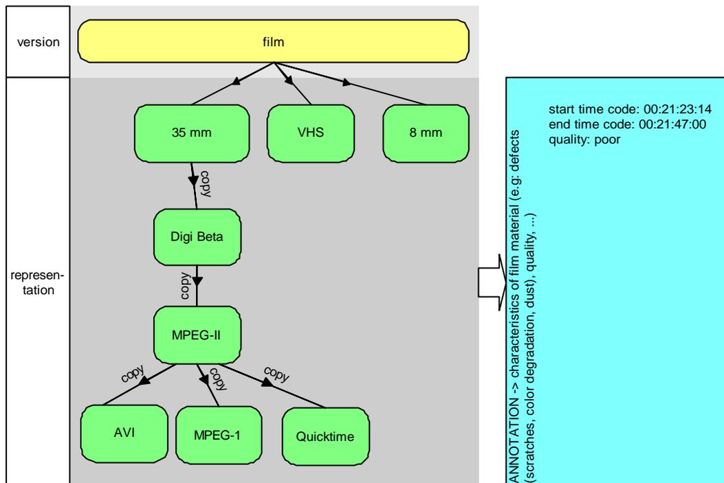
**Figure 2:** Physical representation of an example film
