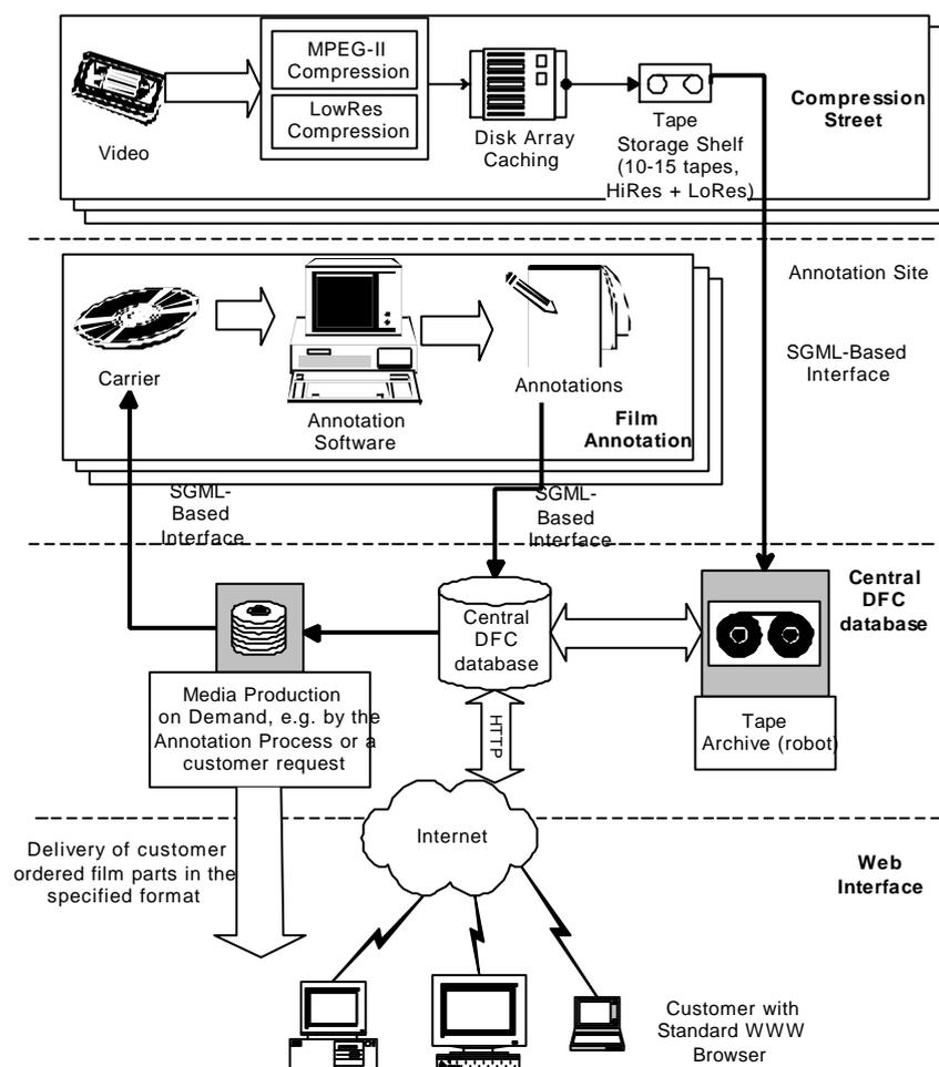
**Figure 1:** High level building blocks of the Digital Film Center
