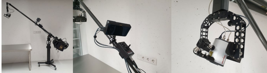
Fig. 4. Crane mounted camera for filming in the dissection rooms
